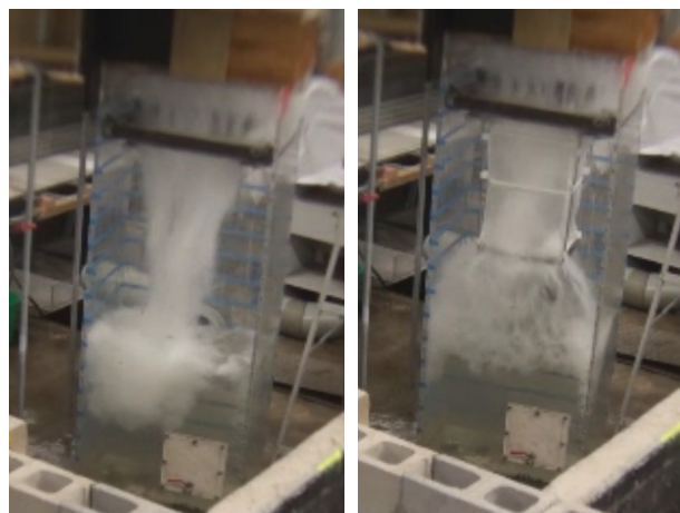
Turbulence in sumped stormwater inlet (left) and EnviroBasin™ (Right)
